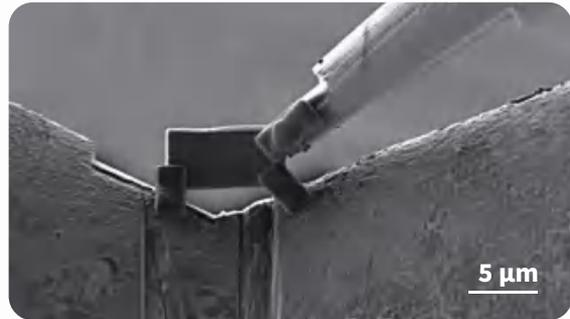
⑥ Weld lamella onto a copper grid
