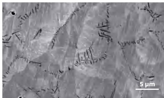
Reinforcement phases in alloy
