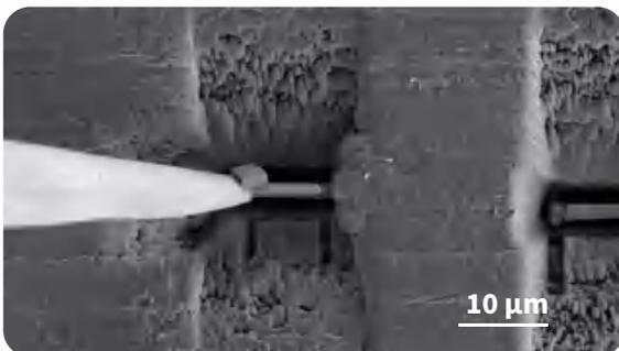
④ Once welded, finish-off of a U-cut prior to lamella lift-out.
