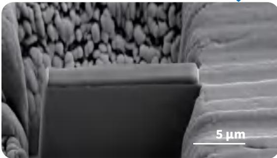
② Rough then precision milling for gross preparation of lamella
