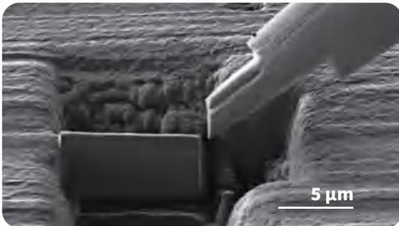
③ Partial separation done on lamella, prior to welding onto a nano-manipulator.
