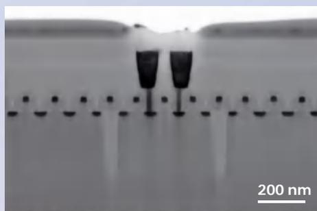
IC Chip device layer Dark-field image (STEM-DF)
