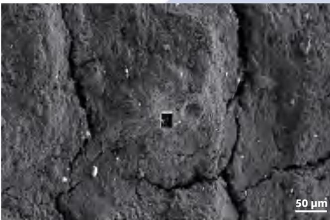
Surface processing location of proton exchange membranes
