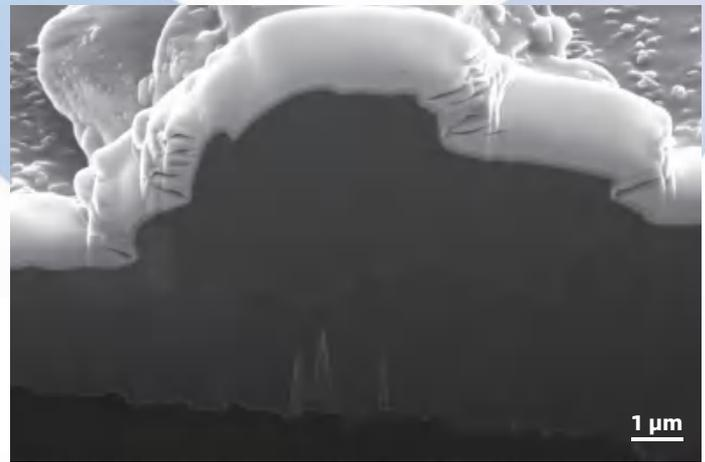
Cross-section of graphite particles
