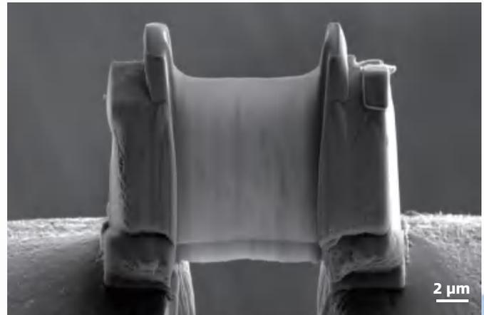
Reinforced phases in titanium metal lamella
