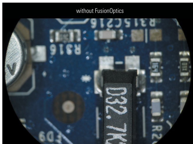
Image simulation, showing a printed circuit board sample without and with the FusionOptics effect, perceived when looking through the oculars.
